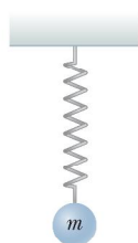
Figure 7.17 (Quick Quiz 7.7) A ball connected to a massless spring suspended vertically. What forms of potential energy are associated with the system when the ball is displaced downward?
