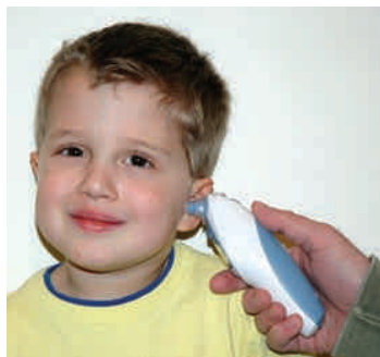
Figure 40.8 An ear thermometer measures a patient's temperature by detecting the intensity of infrared radiation leaving the eardrum.
