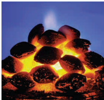
Figure 40.2 The glow emanating from the spaces between these hot charcoal briquettes is, to a close approximation, blackbody radiation. The color of the light depends only on the temperature of the briquettes.
