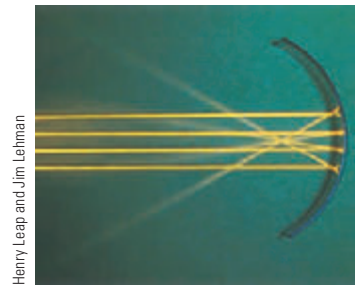
Figure 36.7 Reflection of parallel rays from a concave mirror.
