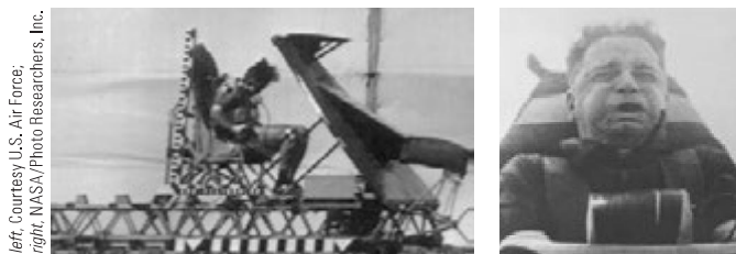
Figure P2.31 (left) Col. John Stapp and his rocket sled are brought to rest in a very short time interval. (right) Stapp's face is contorted by the stress of rapid negative acceleration.
