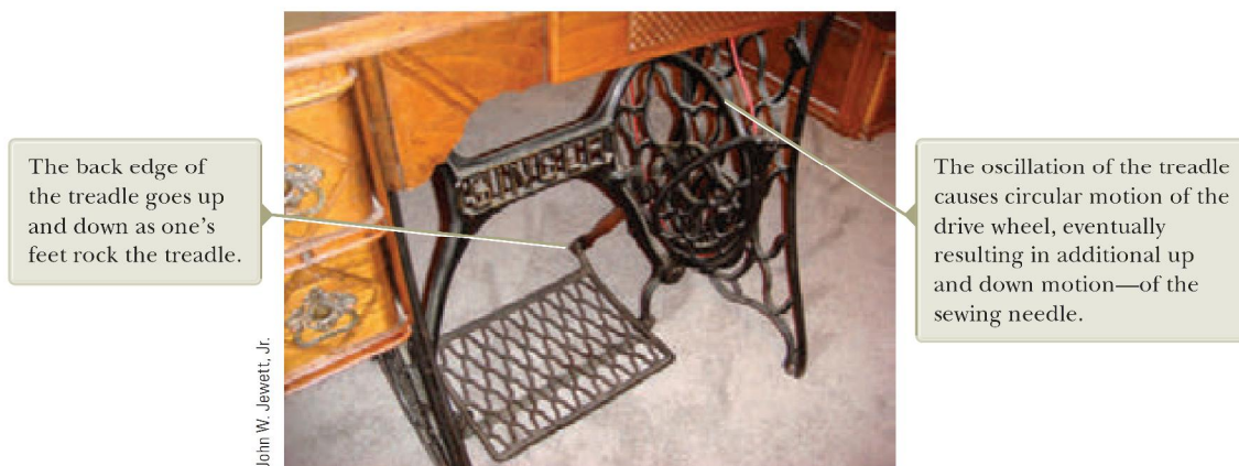
Figure 15.12 The bottom of a treadle-style sewing machine from the early twentieth century. The treadle is the wide, flat foot pedal with the metal grillwork.
