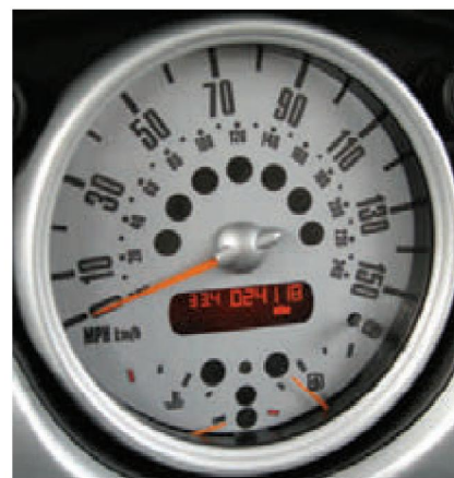
Figure 1.3 The speedometer of a vehicle that shows speeds in both miles per hour and kilometers per hour.
